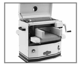
Figure 30. Gauge boards in position.
